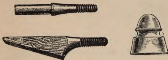
FIGS. 224, 225, 226.—Insulator pin for attaching to cross arm; bracket for attaching to pole or other support; petticoat insulator, to be made of glass or porcelain.
